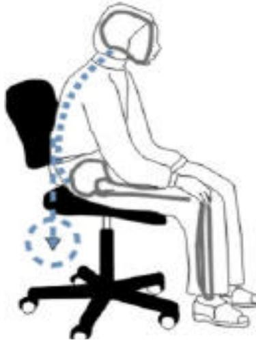
In a conventional seat the centre of gravity is behind the upper trunk.
